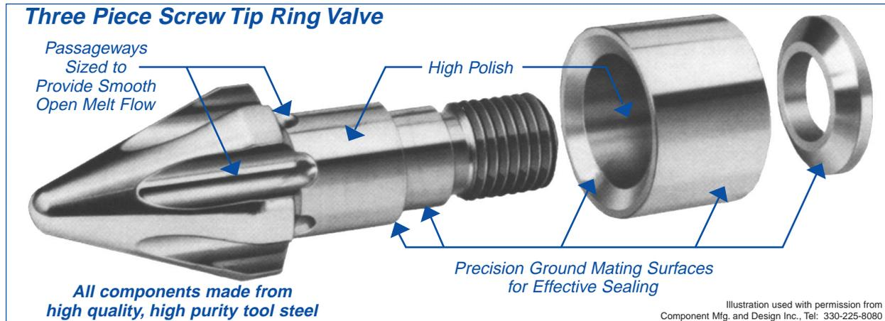
Figure 6 - Disassembled view of a three piece screw tip ring valve assembly showing its component parts
