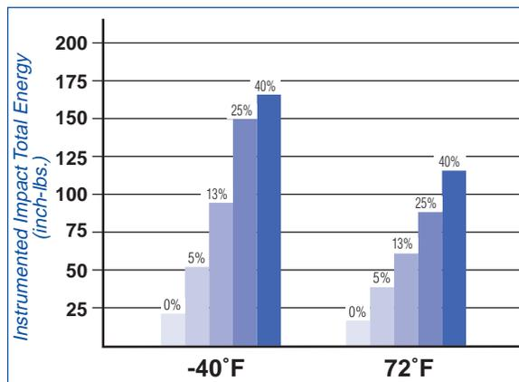
Figure 11 - Impact properties at -40°F and -72°F for unreinforced acetal, acetal blended with Celstran® to 5%, 13%, and 25% glass weights, as well as straight 40% glass Celstran® acetal material.
