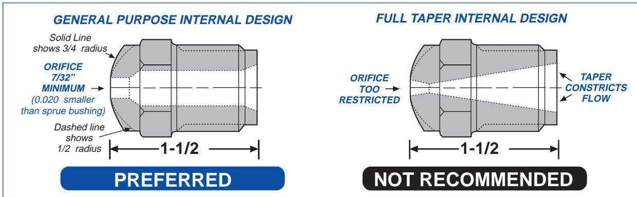
Figure 8 - General purpose and full taper nozzle tips - internal comparison
