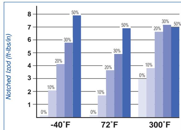
Figure 12 - Notched Izod properties measured at various temperatures for unreinforced polypropylene, and Celstran® long fiber reinforced PP materials at 10%, 20%, 30%, and 50% glass levels.
