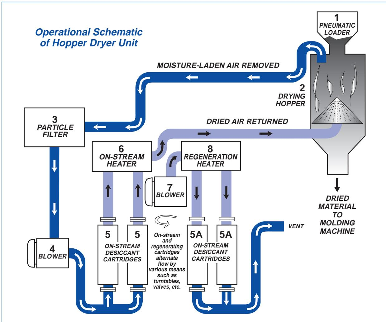
Figure 14 - Hopper dryer unit operational schematic
