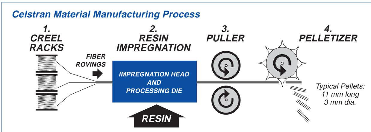
Figure 1 - Polymer Composites Inc. material manufacturing process schematic
