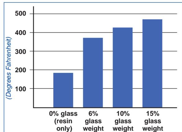
Figure 13 - Deflection Temperature Under Load (DTUL) of recycled, unreinforced PET and as blended to 6%, 10%, and 15% total glass weight with Celstran® PET-GF50-02.
