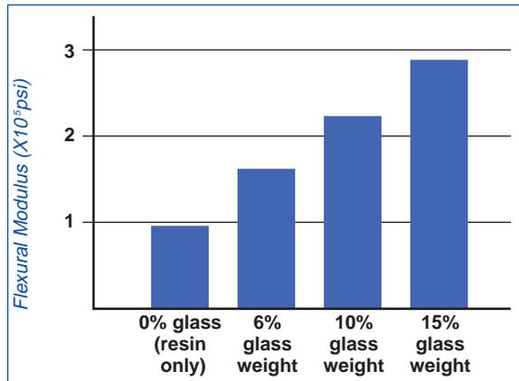
Figure 10 - Flexural modulus of recycled PEHD compared with Celstran® PEHD-GF60-01 blended to total glass weights of 6%, 10%, and 15%.
