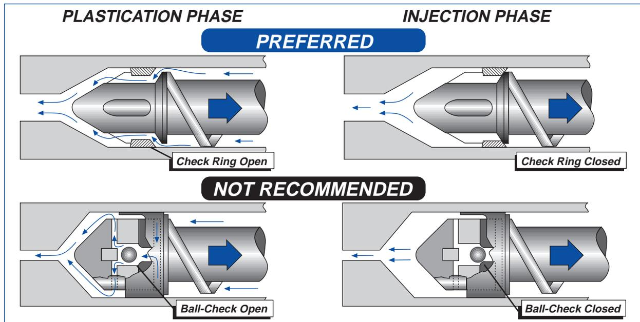
Figure 7 - Preferred check ring non-return valve (above), and not recommended internal ball-check non-return valve (below)
