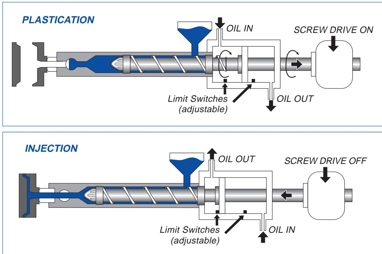
Figure 3 - Molding sequence of a single-stage reciprocating screw injection molding machine.
