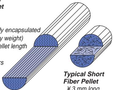
Cutaways show parallel fiber orientation in Celstran vs. random orientation of fibers in short fiber pellets.
